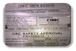
Ensure each container has a manufacture data plate and its up to date.
