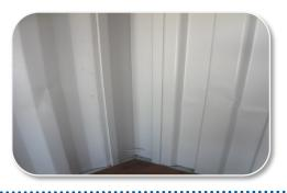
Check corner post and lashing bars to ensure they are free of damage. Broken welds and lashing bars are unacceptable and container should be rejected.
