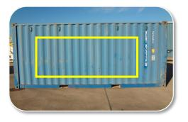
Inspection criteria for side walls will be limited to no more than 4 consecutive creased corruga-tions, no free floating patches, tears, holes in-side marked area of container, will result in re-jection.
