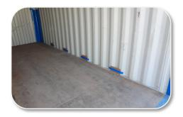
Interior needs to be checked to ensure its in a clean state and free of strong odors. Floor needs to be checked and free from holes, burns, splinters, stains and sharp edges.
