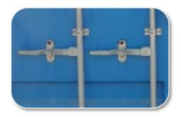
Container needs to have dual locking bars and handles on each door.
